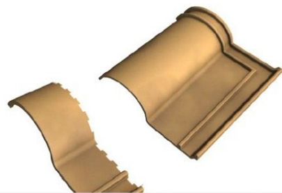
Tiles cutting for top flashing
