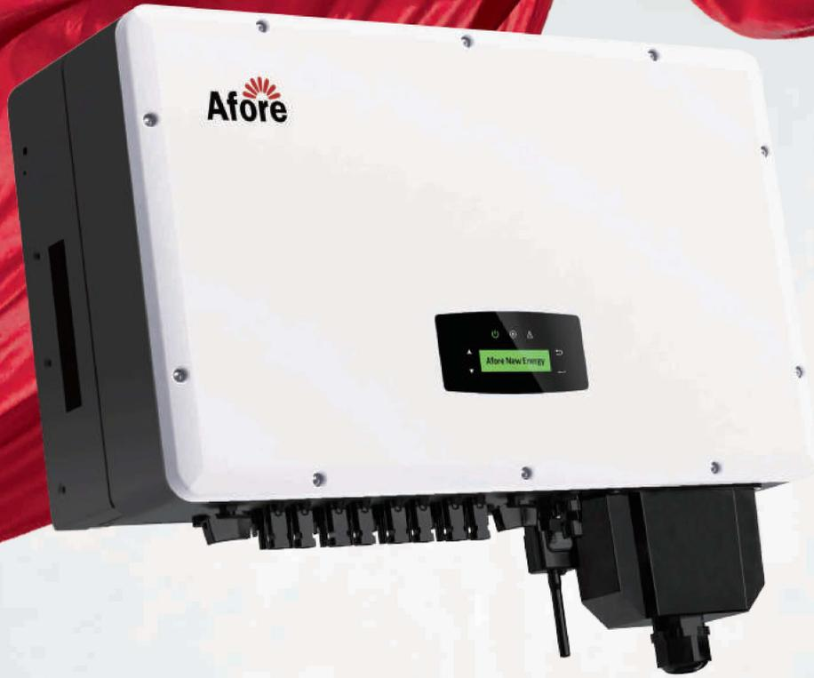
The Afore BNT Series Three-phase string inverters are designed for commercial and power plant PV system applications, rating from 30kW to 60kW. All models with aluminum housings which is anodized, increasing durability and effectively prevents corrosion. Equipped with external inductors, ensure efficient heat dissipation, which significantly improves the reliability and extends the life of the inverters.
